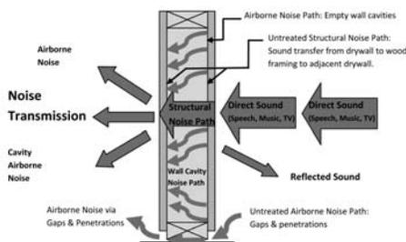
**Figure 1. Noise paths through an Untreated wall assembly.**
