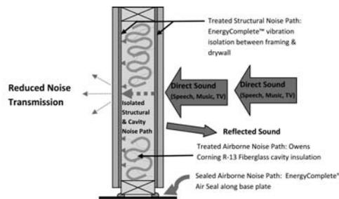
**Figure 2. Reduced noise paths through a Treated wall assembly.**
