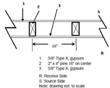
**Figure 3: Base Untreated Interior Wall Assembly**
